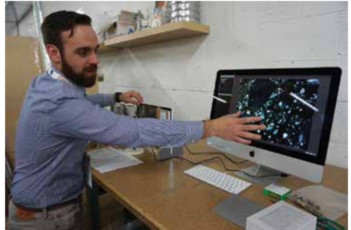
George Reo, WJE, applies a polarizing filter to a petrographic sample to view aggregate color
