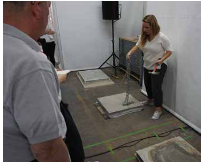
Ann Harrer, WJE, demonstrates NDT methods on concrete samples
