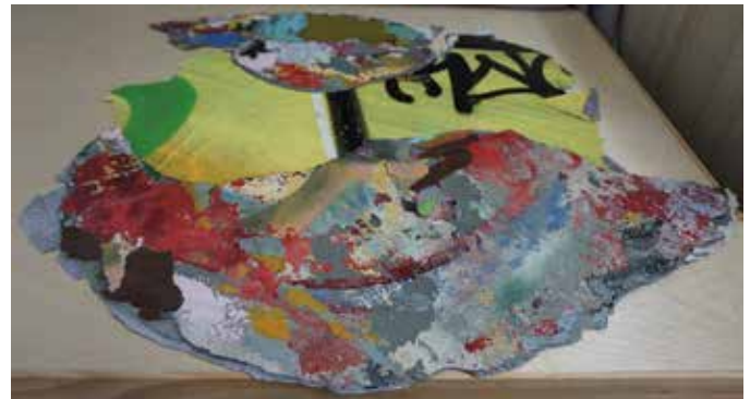
Sample of graffiti and paint layers from the Miami Marine Stadium
